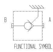
NORMALLY CLOSED CHECK VALVE WITH TOGGLE RELEASE. THE OVER-CENTER TOGGLE WILL HOLD THE VALVE OPEN. AN IDEAL APPLICATION SUGGESTION IS A "TRANSPORT LOCK". THIS CHECK REQUIRES A DIFFERENTIAL OF PRESSURE FROM PORT A TO PORT B TO BE 2:1 OR GREATER WHEN FLOW IS FROM A TO B.
